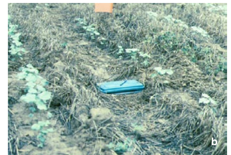
Figure 8. Runoff collectors buried in the middle of crop rows were used to collect sediment in winter fallow/conventional tillage (Figure 8a) and in wheat cover crop/strip-tillage (Figure 8b).
