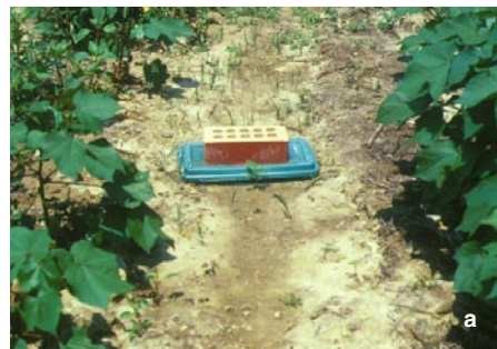
Figure 8. Runoff collectors buried in the middle of crop rows were used to collect sediment in winter fallow/conventional tillage (Figure 8a) and in wheat cover crop/strip-tillage (Figure 8b).
