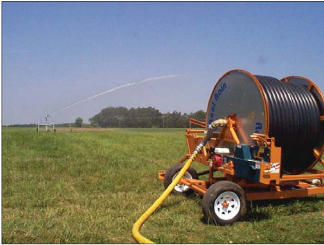
Figure 1. Traveling gun irrigation system. Gun pressure typically ranges from 40 to 80 psi.
