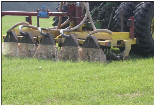
Figure 3. Hosedrag sprayer with 5 nozzles operating at less than 5 psi.
