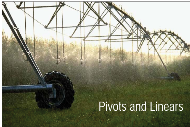
Figure 2. Center pivot or linear move with high-pressure (20-30 psi) drop nozzles.
