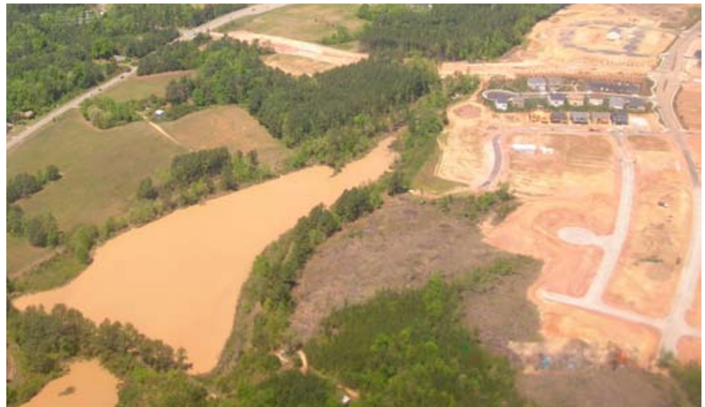
Figure 1. A pond adjacent to a construction site shows the effects of turbidity.
