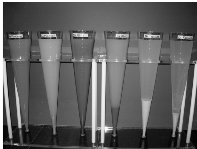
Fig. 1. Floc density studies using Imhoff cones: the clear demarcation between the settled flocs and the suspended sediments was used to calculate the floc density from the volume occupied by the settled flocs.
